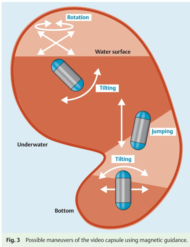
**Fig. 3** Possible maneuvers of the video capsule using magnetic guidance.
