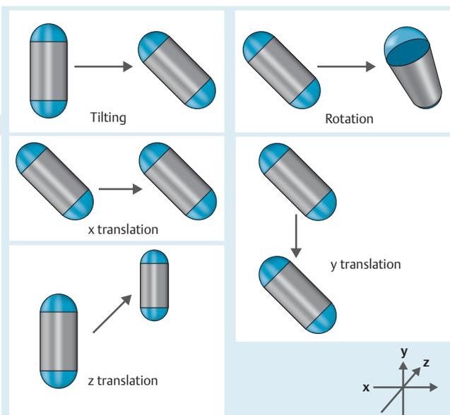
**Fig. 2** The capsule can be magnetically steered with five mechanical degrees of freedom (translation in three dimensions, and rotation and tilting).
